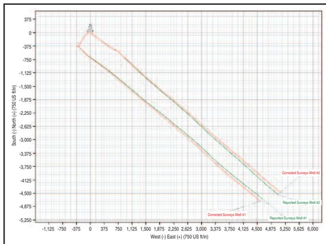
For wellbores that were analyzed after drilling, the difference in position represents how far the bottom-hole locations actually were placed, compared with the original measurements. For wellbores that were evaluated and corrected in real time (the case for the majority of wells), the difference in position represents the distance the bottom-hole location would have been from the plan without applying advanced survey management.
