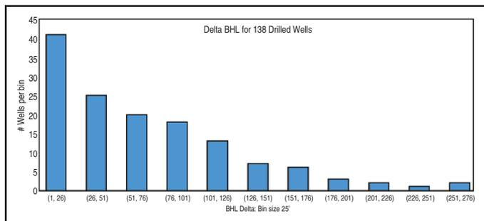
magnetic drill string interference or instrument bias and scale errors using IFR and MSA. After identifying and correcting the systematic errors, the corrected surveys were delivered to the rig site through the Web interface for directional steering.
